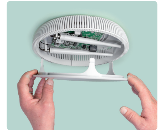
10 Close the cover. Three snap locks shall match the openings on the diameter of the Body.
