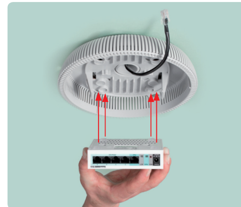
12 Attach the RB751/RB951 to the Mounting Bracket by simple Push and Lock. Device feet shall match exactly to the sockets in the Mounting Bracket.
