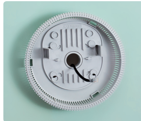
11 Attach the Mounting Bracket to the Body using bayonet lock. Don't forget to pass the cable(s).
